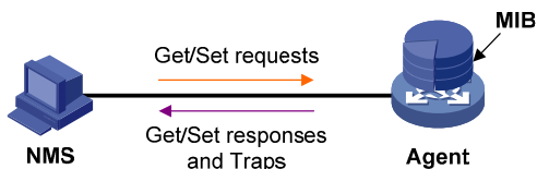
Figure 1-1 Relationship between NMS, agent and MIB
