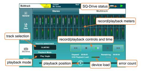
In 96kHz operation the top row of 16 meters is displayed with the bottom row greyed out. When the USB sample rate is set to 48kHz, all 32 meters are shown.
