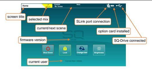
This is the first screen shown when powering on the SQ. It is also shown when no channels are selected, and '**Processing**' or '**Routing**' screen keys are active.
