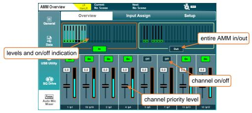
The top part of the screen displays an overview of all AMM slots, with the metering showing gain being applied to channels and indication of whether channels have AMM switched on.
