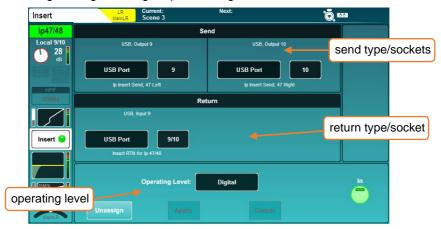
Inserts can also be used with the internal FX engines. See the FX engines section for more details.
