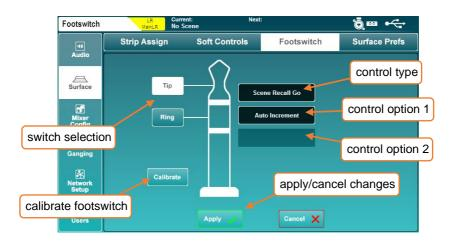
When first connecting a footswitch, touch the 'Calibrate' button to set the type of switch being used. Follow the on-screen instructions.
