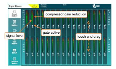
The first four tabs on the 'Meters' screen show 'Input Meters', 'FX Meters', 'Mix Meters' and 'USB Meters'.
