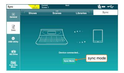
Once in sync mode, pushing and pulling of data is controlled by SQ-MixPad.
