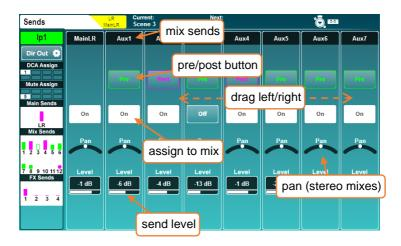
This screen displays all sends and mix assignments for the selected channel.
