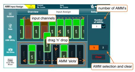
The top part of the screen shows the available input channels and at the bottom are available AMM slots
