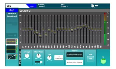
All mix channels feature a 28-band stereo graphic EQ which can be switched in or out by using the on-screen 'In' button.
