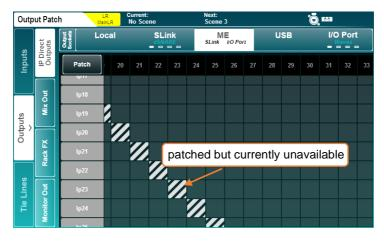
(i) All patching to a currently disconnected device will become active once the device is connected.
