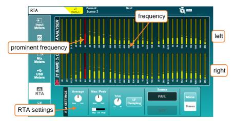
By default, the Meters screen 'RTA Souce' is set to 'PAFL' to match what is being sent to the headphone output and 12 segment LED meter. The source can also be switched to a specific fixed channel if desired.
