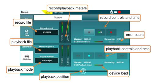
The top half of the screen is for recording and the bottom half is for playback.
