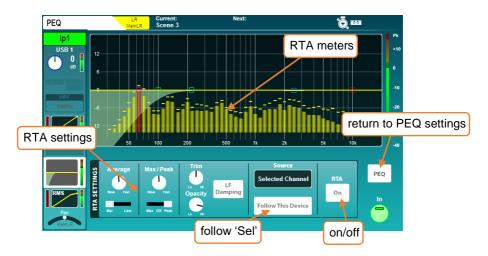
The average meters for the PEQ RTA can either be displayed as bars, with each meter's centre aligned with the frequency it represents, or as a line.
