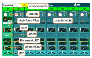
This gives the processing overview for up to 8 channels at once, with the selected channel highlighted. The view will automatically change if a channel is selected which is out of view, though you can also touch and drag to see all channels in the current layer.
