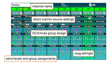
If a channel is assigned to a DCA or Mute group, this is shown with a filled, numbered icon.
