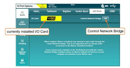
This screen shows which option card is currently connected. It also contains the 'Control Network Bridge' switch.
