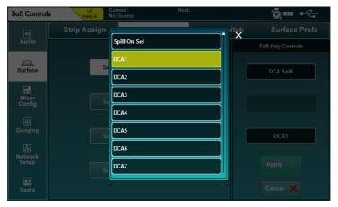
Press the Key to instantly spill the DCA. The SoftKey will flash and the spilled DCA will be shown next to the currently selected mix on screen.
