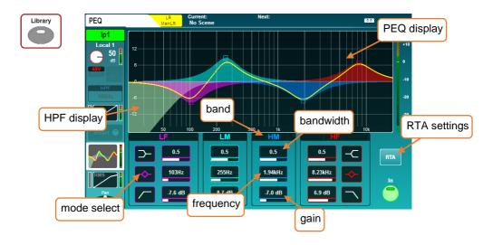
The PEQ can be switched in or out using the physical 'In' key on the surface or with the on-screen 'In' button.
