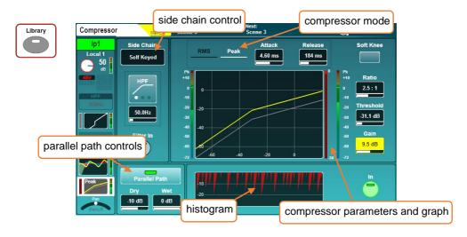
Switch the Compressor in or out using either the on-screen '**In**' button or the physical Compressor '**In**' key (to the left of the dedicated Compressor threshold rotary).
