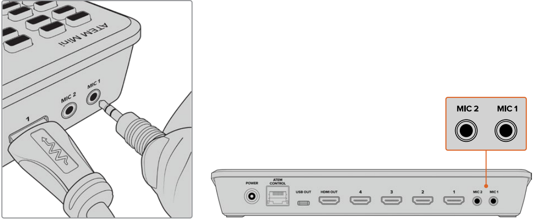
Connect microphones to ATEM Mini's mic inputs
