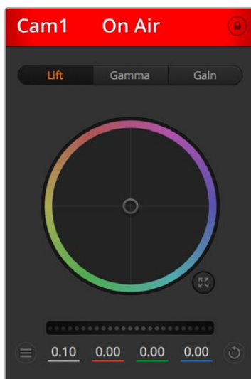
Each camera controller displays the channel status so you know which camera is on air. Use the color wheels to adjust each YRGB channel's lift, gamma and gain settings.
