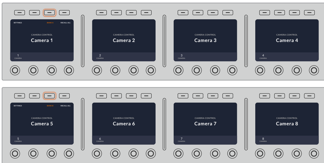
The bank setting lets you assign 2 banks of cameras to the four CCUs and then instantly swap between them by pressing the 'bank' soft button
