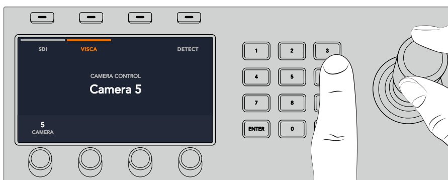
Select the camera you want to control and use the joystick to pan, tilt and zoom
